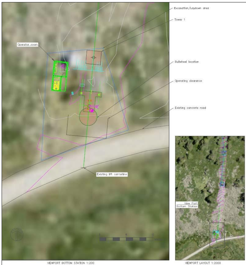
FIGURE 11 BOTTOM STATION LAYOUT
